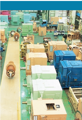
Three-Phase Brushless Synchronous Alternators
